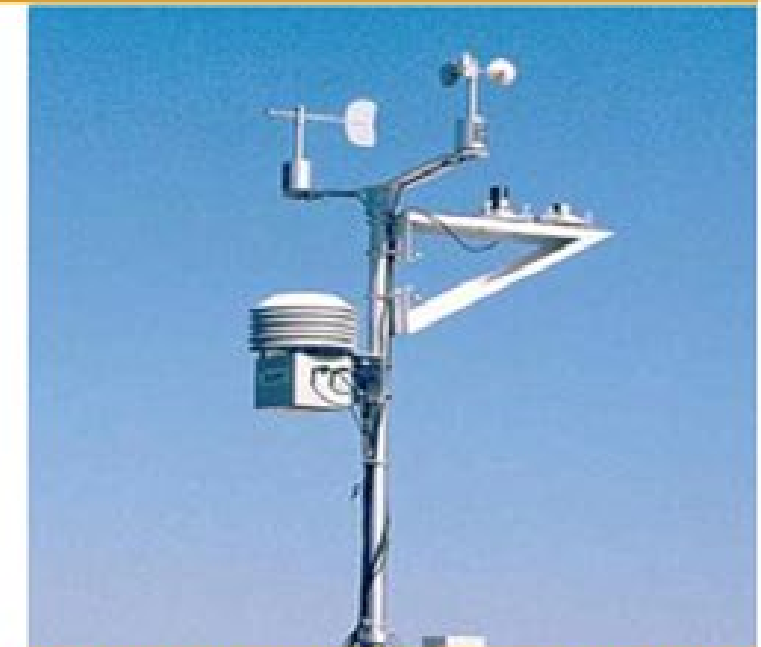
Automatic weather station MiniMet (Skye Instruments Ltd., UK) with DataHog 2 datalogger for signal pro-
