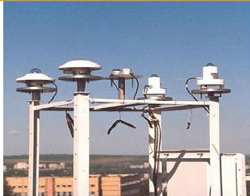
Stationary platform with sensors for global solar radiation measurements and with datalogger CR10X-4M
