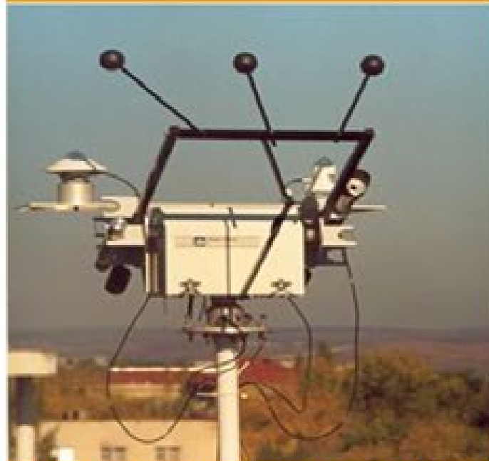
Automatic solar tracking platform 2AP BD (Kipp&Zonen, the Netherlands) with sensors for diffuse
