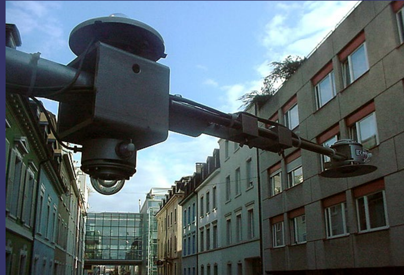
Full radiation components are measured once on top (33m) and also inside the canyon. Here, the system measuring directly over the street level at a height of 3.2m is shown. Photographed towards E. 6.12.01.
