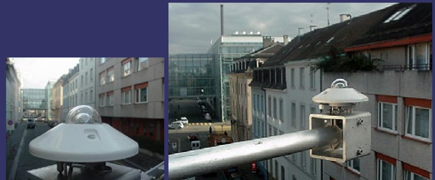
An additional Pyranometer (CM11) below rooftop at 12.4m (z/zH~0.8). Photographed towards E. 6.12.01.
